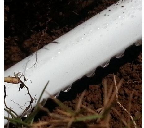
The sweating of water through its micro pores.
